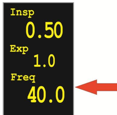
Fig. 75: Version with selectable breathing frequency
