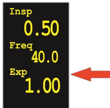
Fig. 74: Version with selectable expiration time
