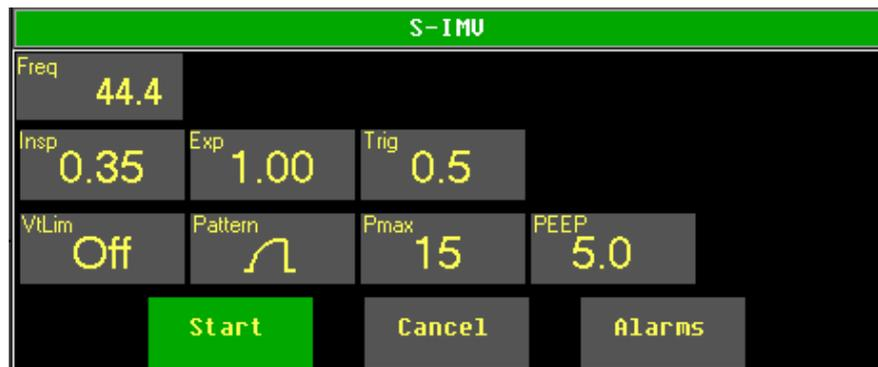
Fig. 62: Starting ventilation
